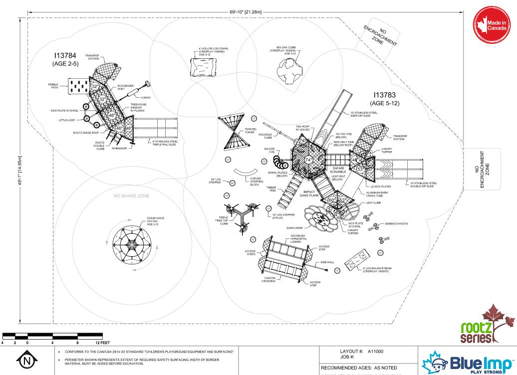
BLUE IMP SLIDES MUST BE INSTALLED WITH SLIDE BEDS FACING BETWEEN NORTH AND EAST
