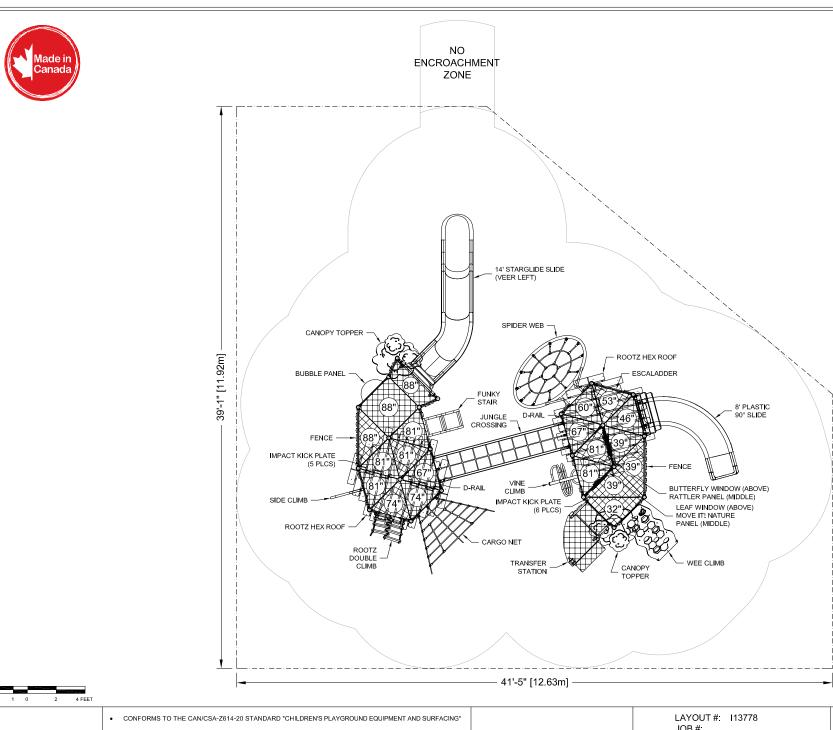
PERIMETER SHOWN REPRESENTS EXTENT OF REQUIRED SAFETY SURFACING. WIDTH OF BORDER MATERIAL MUST BE ADDED BEFORE EXCAVATION.
