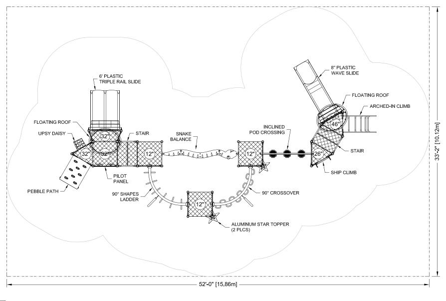
BLUE IMP RECOMMENDS THAT SLIDES BE INSTALLED WITH SLIDE BEDS FACING BETWEEN NORTH AND EAST CONFORMS TO THE CAN/CSA-Z614-20 STANDARD "CHILDREN'S PLAYGROUND EQUIPMENT AND SURFACING"
