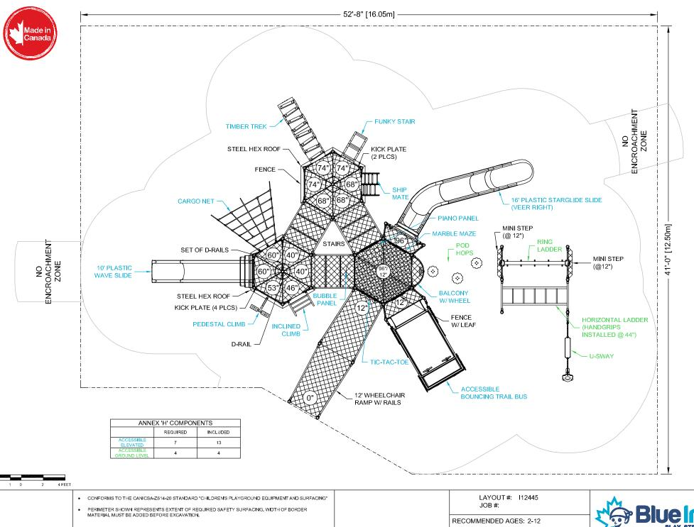
BLUE IMP RECOMMENDS THAT SLIDES BE INSTALLED WITH SLIDE BEDS FACING BETWEEN NORTH AND EAST
